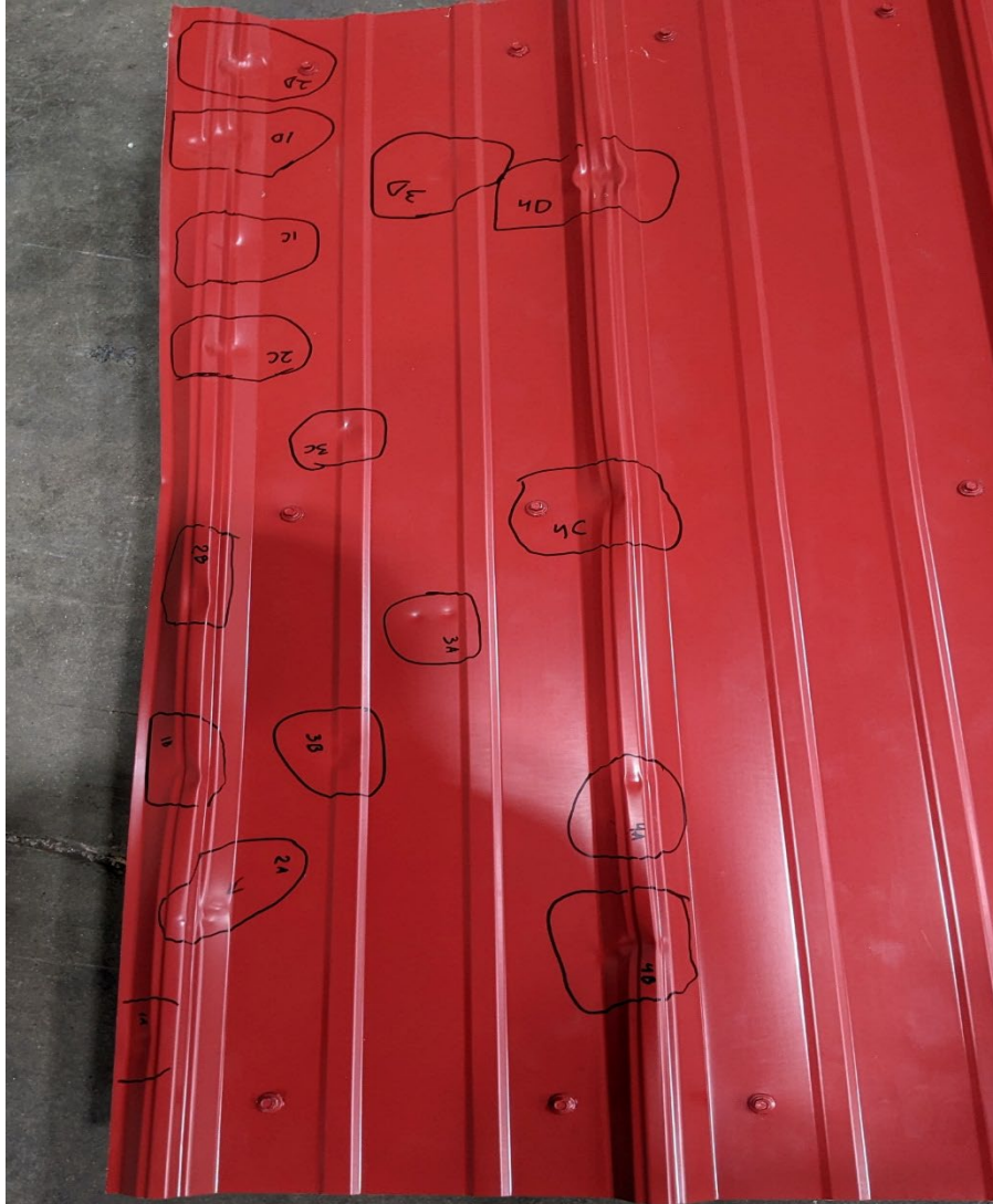
Photo No. 2 Impact locations detail
