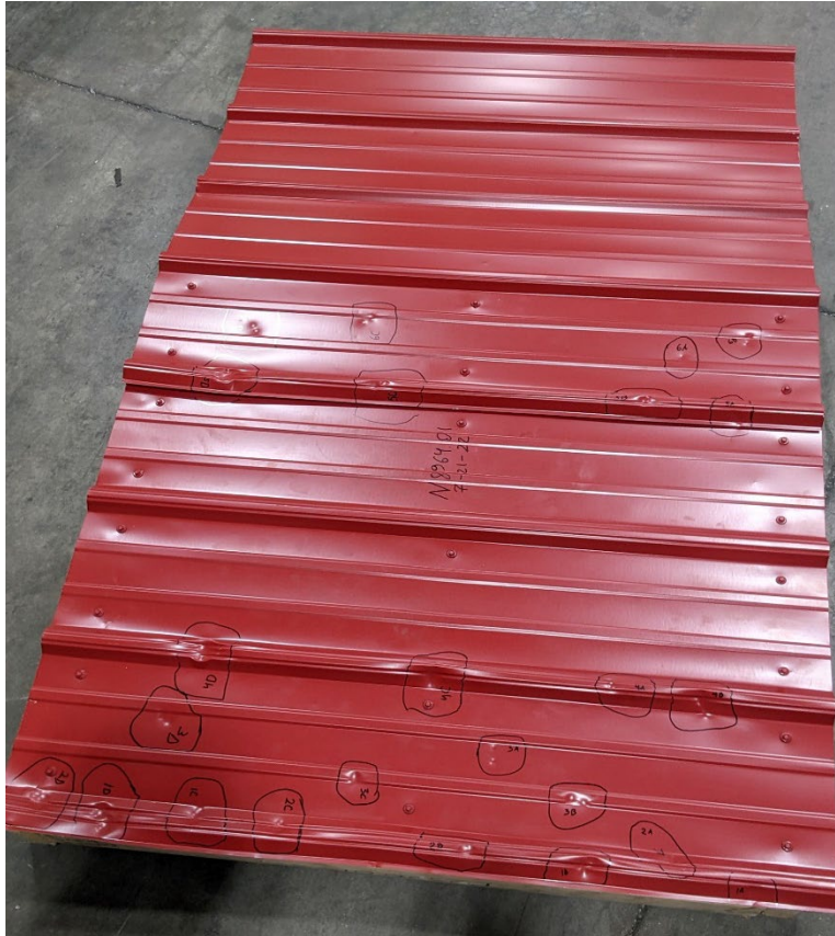
Photo No. 1 Test setup and overall impact locations.
