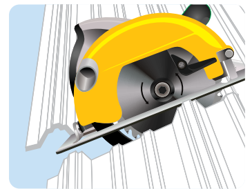
Sawing the panels Figure 4
